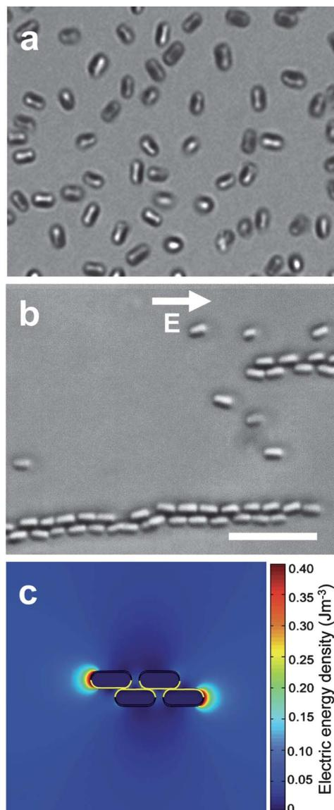
**Fig. 3** Bright-field microscopy images of (a) side-coated Janus rods in absence of an electric field and (b) staggered chains composed of side-coated Janus rods assembled parallel to the electric field direction at  $15 \text{ V mm}^{-1}$ ,  $100 \text{ kHz}$ . The scale bar is  $10 \mu\text{m}$ . (c) Finite element modeling of electric energy density ( $\text{Jm}^{-3}$ ) distribution around overlapping staggered side-coated Janus chain at  $15 \text{ V mm}^{-1}$ ,  $100 \text{ kHz}$ .
