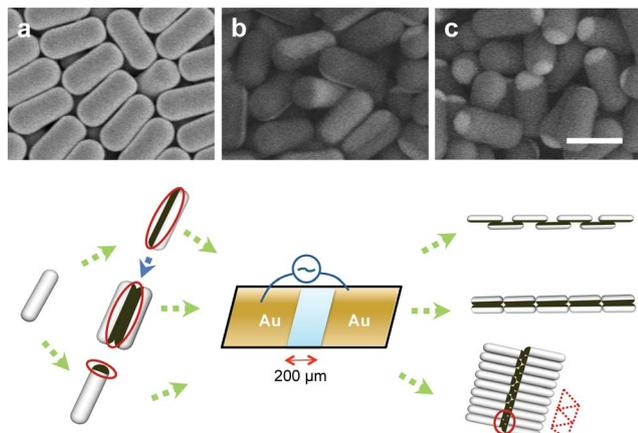
Fig. 1 SEM images of (a) homogeneous silica rods ( $L/D = 2.1$ ), (b) side-coated Janus rods, and (c) tip-coated Janus rods (or matchsticks). The scale bar is 2  $\mu\text{m}$ . (d) Schematic illustration of potential pathways for assembling these patchy particles into chain-like structures in an AC electric field.
