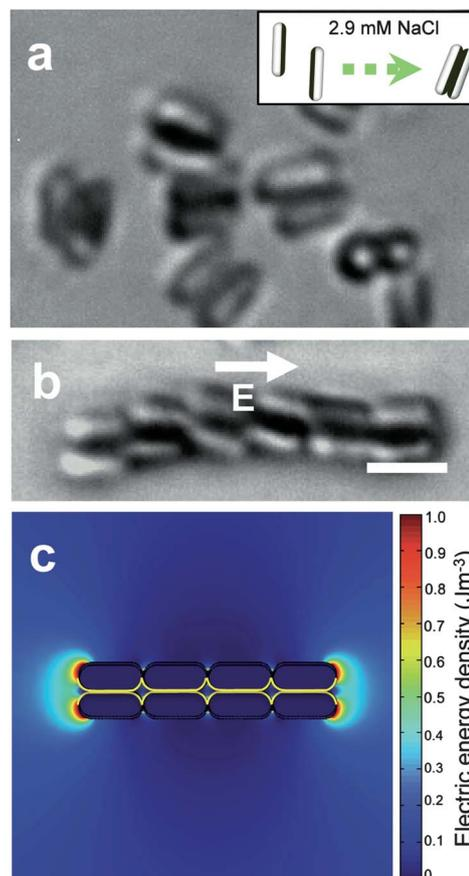
**Fig. 4** (a) Janus rod doublets are formed by side-coated Janus rods with the addition of  $2.9 \text{ mM NaCl}$ . The inset shows the formation of Janus doublets from side-coated Janus rods. (b) A flexible doublet chain assembles parallel to the electric field direction at  $20 \text{ V mm}^{-1}$ ,  $100 \text{ kHz}$ . The scale bar is  $3 \mu\text{m}$ . (c) Finite element modeling of electric energy density ( $\text{Jm}^{-3}$ ) distribution around a chain assembled from Janus doublets.
