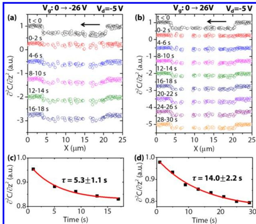
**Figure 6.** Capacitance ( $\partial^2 C/\partial z^2$ ) dynamics at  $V_d = -5$  V, following application of a gate bias step of  $\mp 26$  V: (a,b) hole and electron dynamics, and each curve corresponds to the surface potential profile covering the source (left), channel (middle), and drain (right). The tip was scanned from right to left. (c,d) Average  $\partial^2 C/\partial z^2$  in the channel region as a function of time. Black dots are raw data and red lines are exponential fits.
