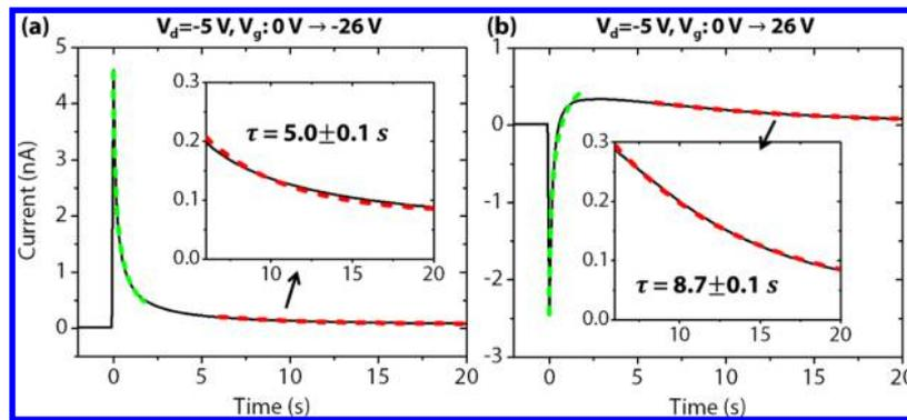
**Figure 4.** Current injection and transport dynamics at a drain bias of  $V_d = -5$  V, after the application of a gate bias step from zero to  $\mp 26$  V, as labeled: (a,b) hole and electron dynamics. Insets are expansions of the curves in the 6–20 s time window.
