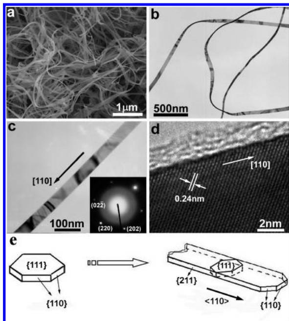
**Figure 1.** SEM (a), TEM (b,c), and HRTEM (d) images of gold nanobelts obtained at 4 °C. (e) Schematic illustration of the growth direction of gold nanobelts. (Inset) ED pattern corresponding to the whole region of c.
